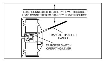
9. Turn **ON** the utility power supply to the transfer switch using the means provided (such as utility main line circuit breaker) or supplementary 70 amp circuit breaker you have installed in the main panel.
